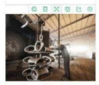
Clean And Heat Treat After the molten metal is poured and solidified, the molding sand is removed, and the gate and other attachments are knocked out to form the required casting.
