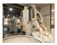
Shell Preparation The workshop has 4 automatic production lines, able to produce 1800 sets of shells. We use hygrothermograph, aerometer, and PH to monitor humidity, temperature, and concentration of liquor aluminum chloride.
